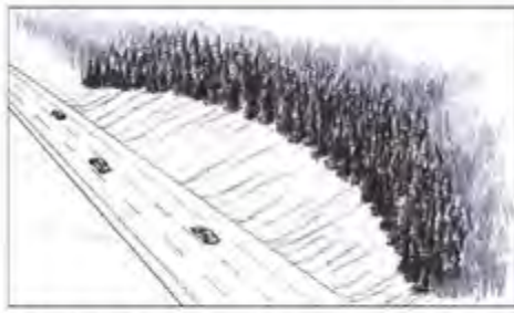
D) Uniform clearing lines create an unnatural edge.
