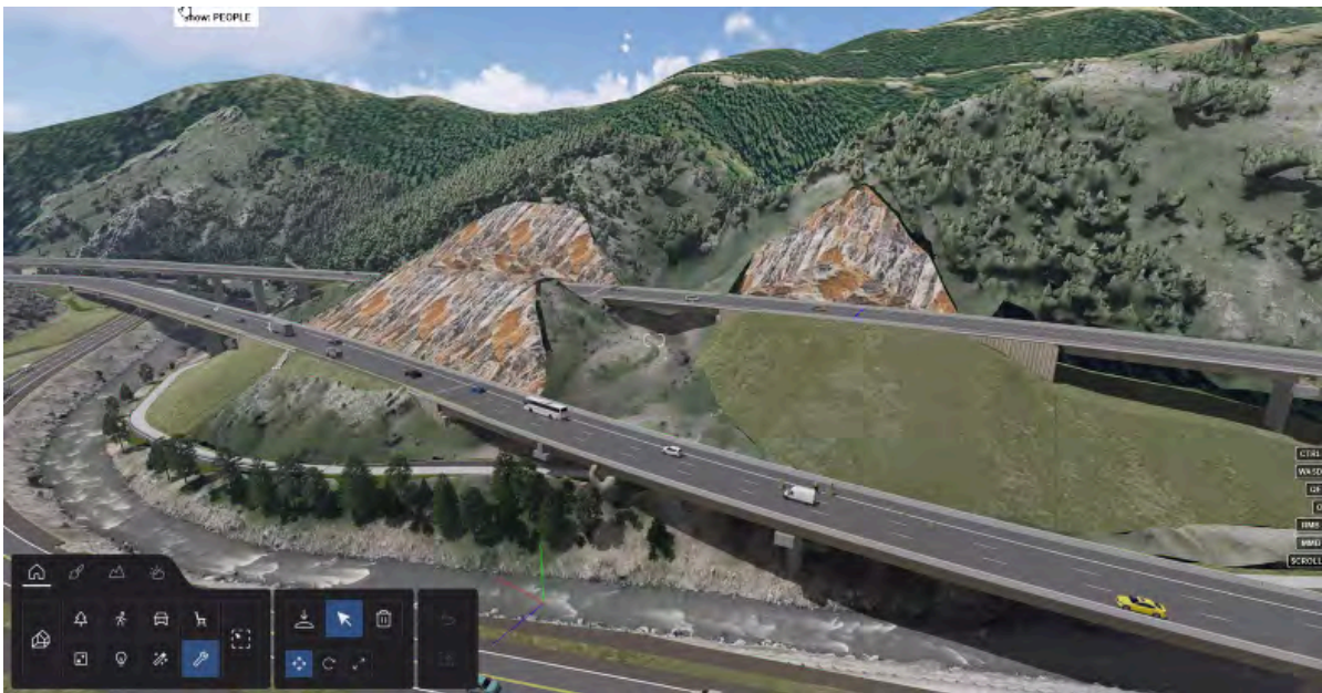
Rendering showing the area with the future Saddle Cut, roadway, and the fill area.
